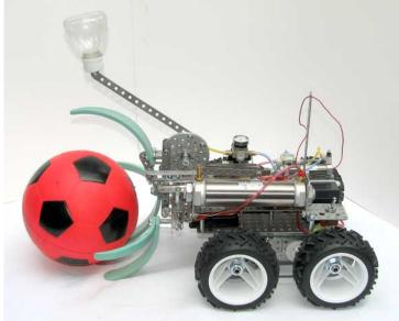
The bot on the left is designed to grasp and lift footballs and soccer balls. This is a game-playing robot suitable for use on a hard packed or asphalt driveway or any indoor floor surface.
